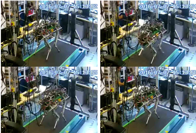
Fig. 2. Push recovery with state estimation in the loop. The robot was commanded to trot in place and keep its position. After several pushes from the operator, the robot recovered its position along the green line of the treadmill. The ability to recover its position in a constrained space using the state estimation in the loop demonstrates the reliability and robustness of the filter.
