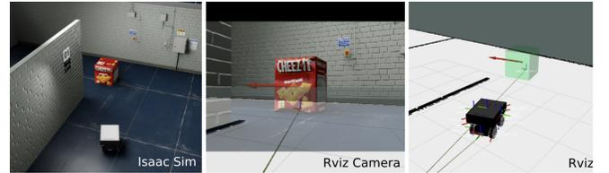
Fig. 4: Obstacle detection and 3D pose estimation, based on DOPE. From left to right: obstacle as placed in simulation, object pose estimation in Isaac Sim, and obstacle in the map.
