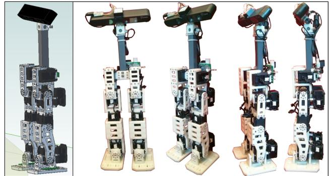
Fig. 1. RPBP: the Rapid-Prototyped BiPedal robot in simulation (left) and the physical in different angles.
