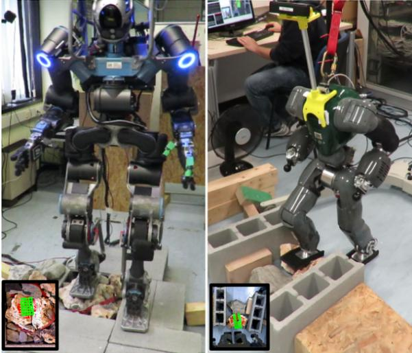
Fig. 11. WALK-MAN and COMAN humanoid robots, using SPL for finding contact patches (in green) onto rocks and stepping on them [18].
