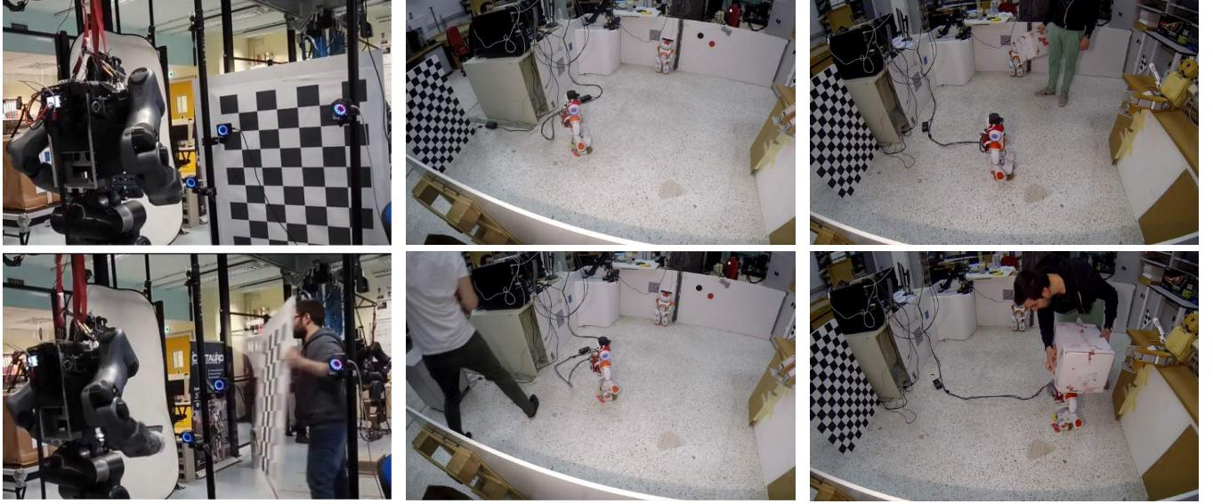
Fig. 2. Illustration of conducted experiments – **Left:** WALK-MAN v2.0 and VO outliers, **Middle:** NAO and VO outliers, **Right:** NAO and LO outliers.
