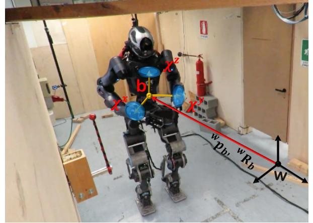
Fig. 1. Illustration of frames used in base estimation on the 29DoF WALK-MAN v2.0 humanoid robot:  $w$  corresponds to the inertial world frame,  $b$  is the base frame, and blue ellipses indicate orientation uncertainty.
