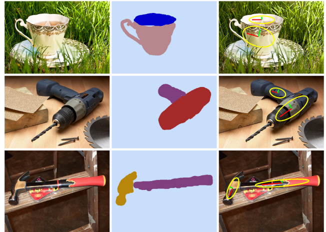
Fig. 1. Object affordances and their grasp frames. From left to right: The original images, the affordances associated with each object in the images, and the grasp frames generated from the affordances.
