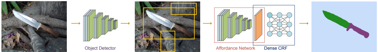
Fig. 2. An overview of our affordance detection method. From left to right: A deep network is first used as an object detector to generate the object bounding boxes that narrow down the region of interest. A second network is then used to produce feature maps from these bounding boxes. Finally, these maps are post-processed with dense CRF to improve the prediction along the class boundaries.
