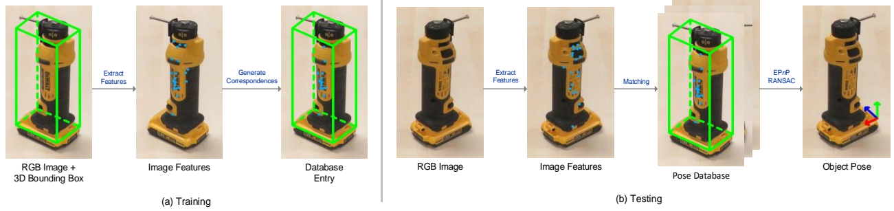
Fig. 3. The pose estimation method. (a) Training : For each image the features are first extracted from the object, then the correspondences between the 2D features and their associated points in 3D space are generated using the predefined bounding box. (b) Testing : The detected features are matched with all the features in the database. The matched correspondences will be used to compute the object pose.
