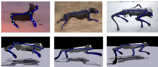
Fig. 5: ViTPose++ Pose Estimation on (top) the demonstration video and (bottom) the training sample.
