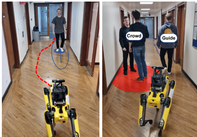
Fig. 1: Social navigation examples, based on the Augmented Social Force Model (ASFM), handling oncoming pedestrians (left) and following people through crowded areas (right).
