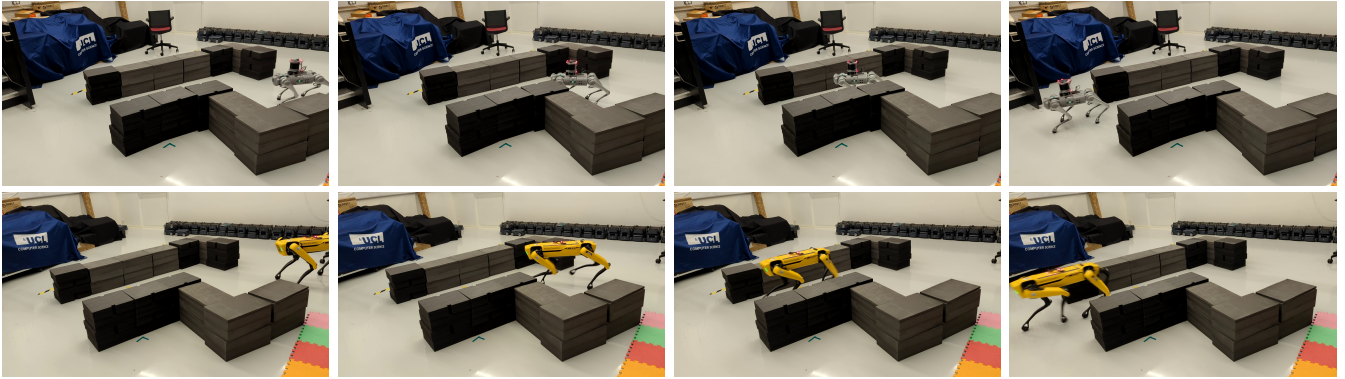
Fig. 5: From left to right we show a sequence of the Unitree Go1 (top) and Boston Dynamics Spot (bottom) robots navigating around obstacles using the ViT- A^* driven navigation stack.
