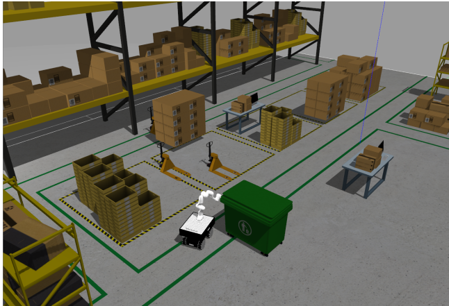
FIGURE 1. The case where a mobile robot following an inspection path (inside the green lines), unexpectedly detects an obstacle that needs to be pushed towards a storage space to clear and free the path.
