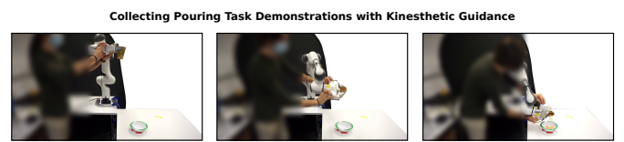
Fig. 5. Collecting pouring task demonstrations via kinesthetic guidance on the Franka Emika Panda robot.
