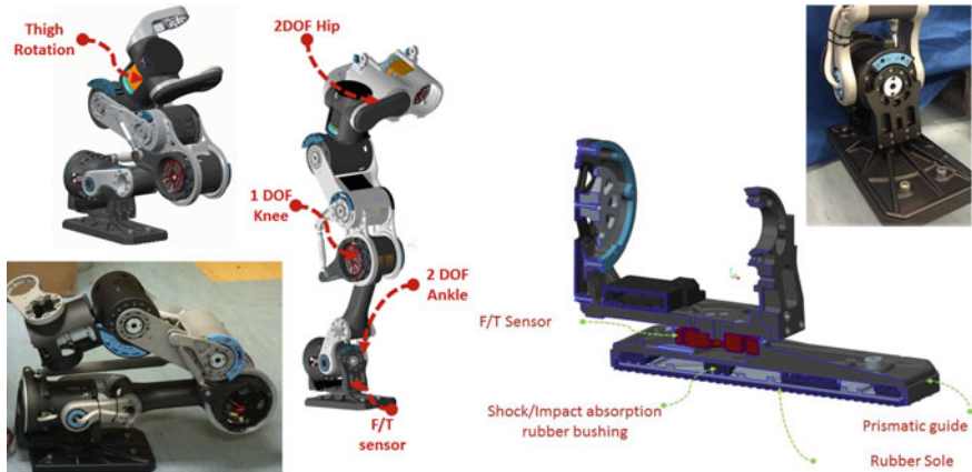
Fig. 9 WALK-MAN leg kinematics and foot design
